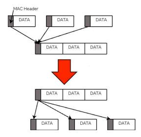
Data can be combined into larger frames to save header overhead.
