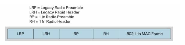
Greenfield is for all 802.11n compatible devices. Mixed mode is when 802.11a/b/g devices are also present.
