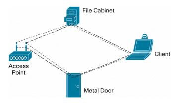
The technique of transmitting data via parallel channels over multiple antennas to create different data paths is called space division multiplexing.
