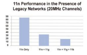
This drops by almost 50% if an 802.11g station is causing congestion in the network. The performance is cut by almost 75% if there is an 802.11b station causing congestion
