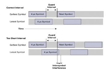
Shortening the guard interval can improve throughput, but intersymbol interference will degrade the SNR
