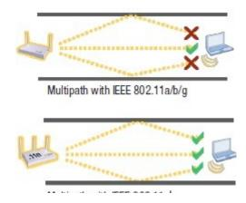
With MIMO technology, the message can be easily reorganised, and actually use multipath reflections to gain signal strength and thus improve reliability. This leads to a greater coverage area for a given data rate, or higher data rates for a given coverage area and more bandwidth.
