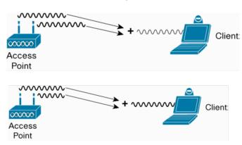
Beam forming can improve the throughput when further away form the AP, but cannot increase the coverage area
