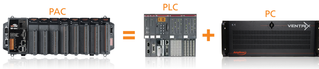
Image 1 - A PAC unit offers the capabilities found in a PLC plus the benefits of an IPC
